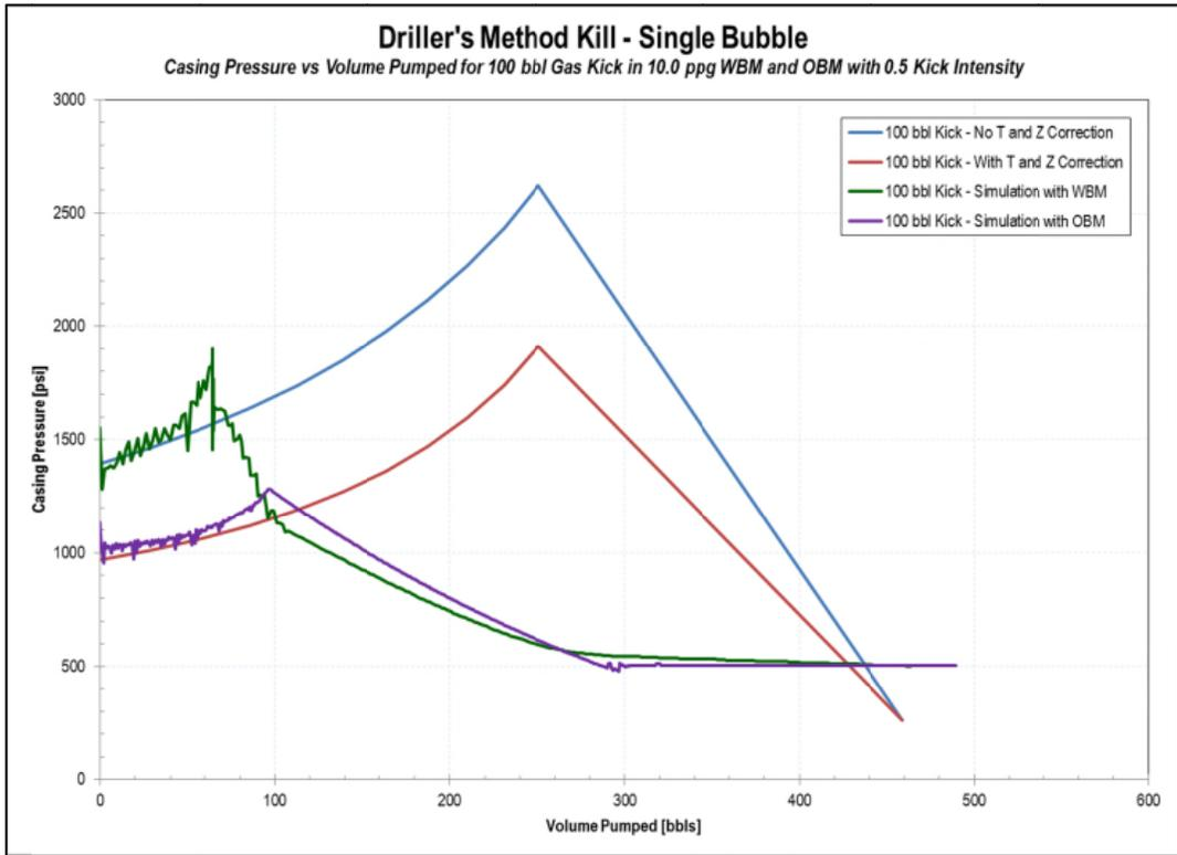
**Figure 2 – Driller's Method Comparison for 100 bbl Kick Volume**
