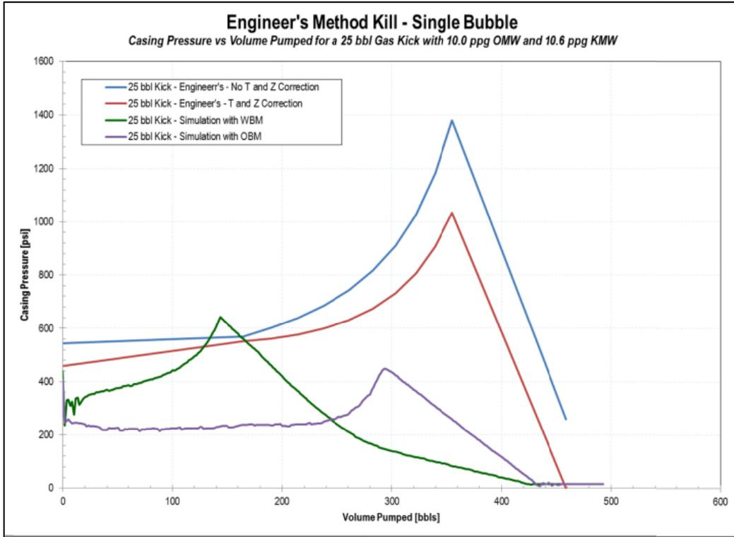
**Figure 3 – Engineer's Method Comparison for 25 bbl Kick Volume**
