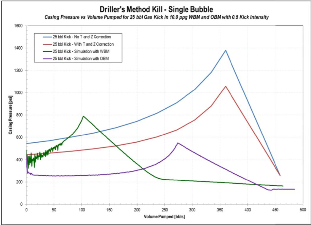
**Figure 1 – Driller's Method Comparison for 25 bbl Kick Volume**
